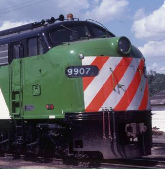
Rapido once again breaks new ground by announcing a first in plastic! Behold the HEP-equipped E-unit, used predominately in commuter and inter-city services. Perhaps the most famous owner was the BN, with a fleet of 25 Morrison-Knudsen rebuilt E-9As for "suburban" service. Notable upgrades included; new 645EC prime movers pushing the horsepower output to 2400, Detroit Diesel HEP generators and the addition of dynamic brakes. The fleet would remain in service until the early '90s.
